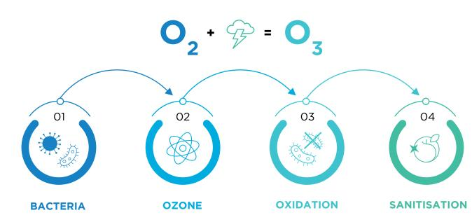
The air in which oxygen is dissolved carries many organic elements such as viruses, bacteria, fungi and allergens Ozone is a very unstable moleculte and rapidly decomposes to release oxygen atoms This single oxygen atom is a powerful oxidising agent that reacts with bad odours, fungus, bacteria and viruses In this way the air is quickly sanitised, leaving the treated area free to be used as normal
