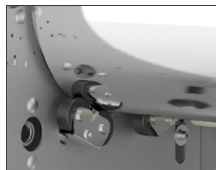
Cylinder Floating Support System.
